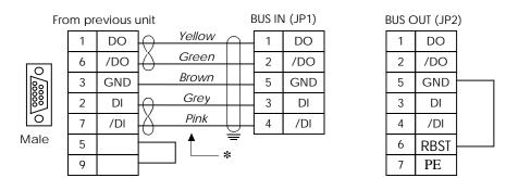
Fig. 5 Installation of the RBST signal
