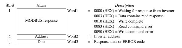
If a fault occurs, the option card indicates an ERROR response by setting the MSB bit in the MODBUS Response code to one (1). The data word then contains the ERROR code.
