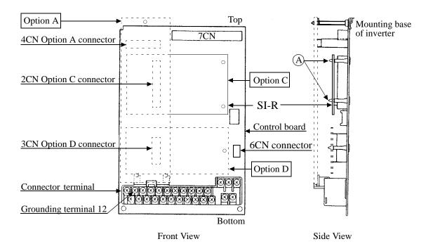
Fig. 2 Installation of the InterBus-S Control Card SI-R
