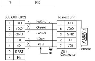
Fig. 4 Wiring of the InterBus-S Control Card SI-R
